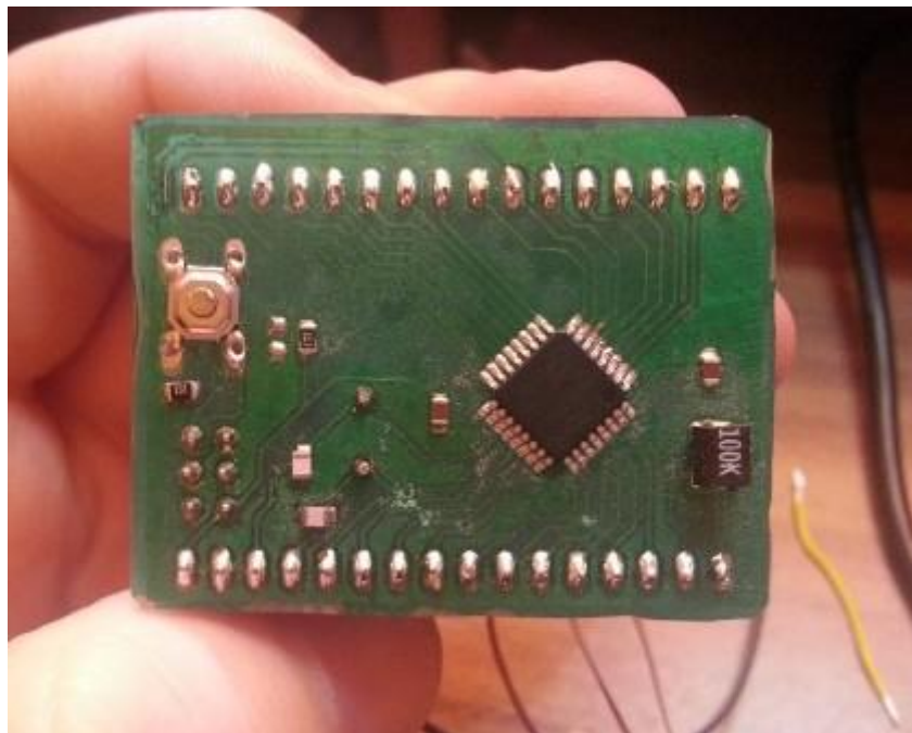
Figure A-3 Manufactured breakout board
