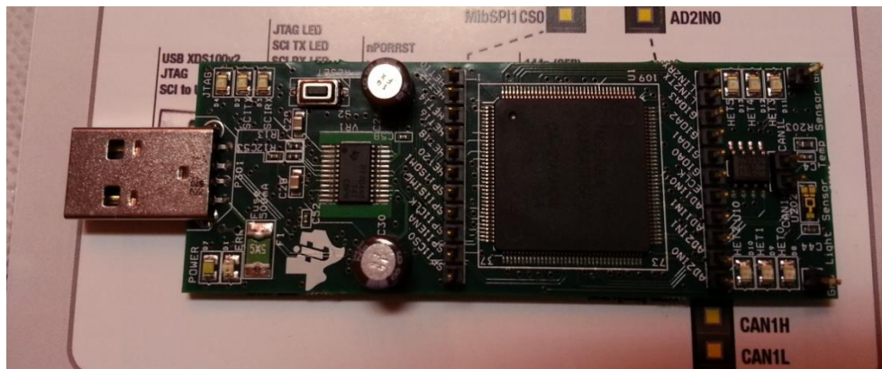
Figure A-1 Texas Instruments TMS570 Hercules family development kit
